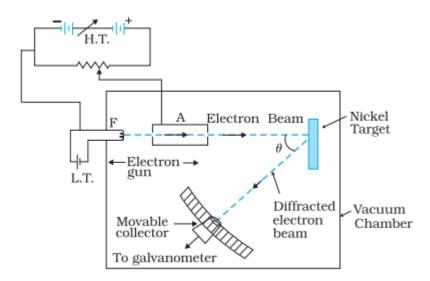
by applying suitable potential/voltage from a high voltage power supply (H.T. or battery). They are made to pass through a cylinder with fine holes along its axis, producing a fine collimated beam.
