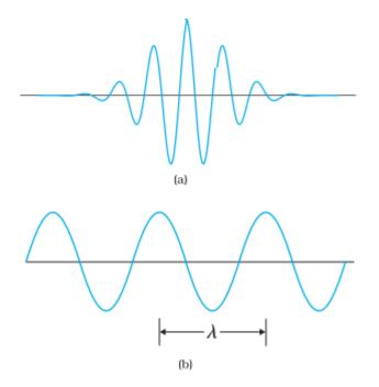
(a) The wave packet description of an electron. The wave packet corresponds to a spread of wavelength around some central wavelength (and hence by de Broglie
