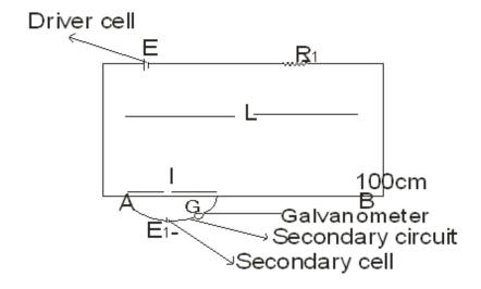
AB is the potentiometer wire; connect the driver cell across it, using suitable resistance from the resistance box
