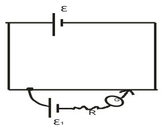
• A resistance in parallel to secondary cell affects the balance point because it draws current from the secondary cell.
