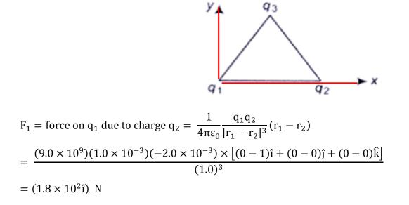
$$F_{2} = \text{force on } q_{1} \text{ due to charge } q_{3} = \frac{1}{4\pi\epsilon_{0}} \frac{q_{1}q_{3}}{|r_{1} - r_{3}|^{3}} (r_{1} - r_{3})$$
