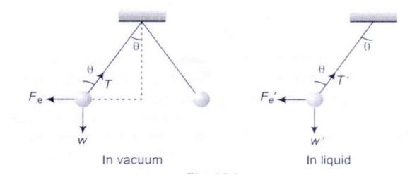
In the liquid,  $F_e' = \frac{F_e}{k}$  where k is dielectric constant of liquid And w' = w - upthrust
