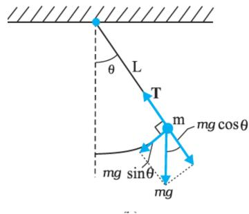
The radial force T-mg cos  $\theta$  provides centripetal force. The tangential force mg sin  $\theta$  provides the restoring force
