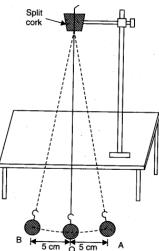
Experimental set up to study the dissipation of energy of an oscillating pendulum
