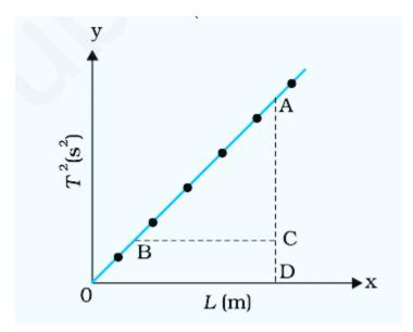
Value of time period for any length can be obtained directly from the graph also we can obtain the length of the pendulum if we know its time period
