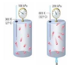
https://image.slidesharecdn.com/p141n2gaslawkmt-100112100040phpapp02/95/lecture-141-142-gas-laws-kmt-21-728.jpg?cb=1263836694 Figure shows that the pressure in the cylinder doubles (100kPa to 200kPa) when the temperature (in kelvin) increases to twice its original value (300K to 600K).
