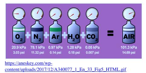
The figure above shows that the total pressure of 101.3 kPa exerted by the atmosphere is equal to the sum of the individual pressure of the component gases which make up the air.
