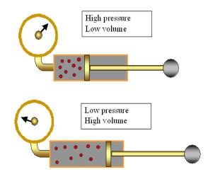
Figure shows the expansion of a gas in a cylinder when the piston is pulled out. The pressure decrease as the volume increases
