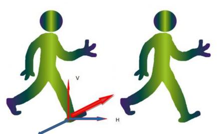
The reaction force R can be resolved into two components: vertical component V and horizontal component H.
