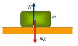
But these are not third law pair of forces, because here both the forces are acting on the same object (block). Whereas, according to third law, pair of forces must be exerted on two different blocks.
