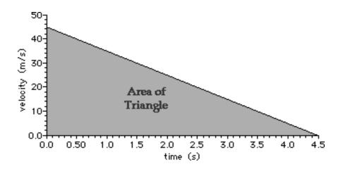
(b)The distance travelled can be found by a calculation of the area under the velocity time graph
