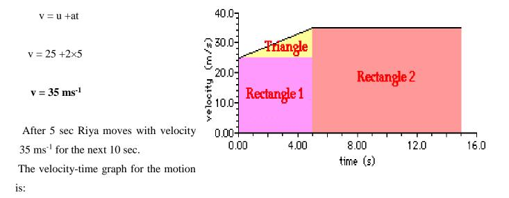
(b) The distance travelled can be found by a calculation of the area under the velocity time graph.
