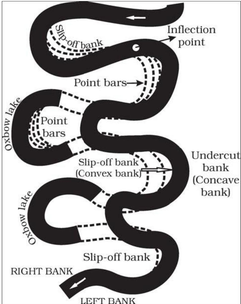
Figure 12a : Meander growth and cut-off loops and slip-off and undercut banks
